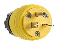
Rated watertight for 1,500 psi high-pressure hosedown, Pass and Seymour plugs and connectors feature multiple seals to ensure protection against the environment. Constructed of a sturdy rubber body, which makes them impact- and chemical-resistant, they have nickel-plated blades and contacts for superior corrosion resistance.
