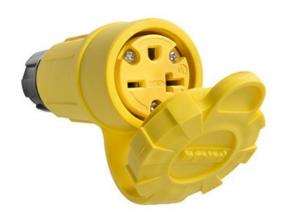
Rated watertight for 1,500 psi high-pressure hosedown, Pass and Seymour plugs and connectors feature multiple seals to ensure protection against the environment. Constructed of a sturdy rubber body, which makes them impact- and chemical-resistant, they have nickel-plated blades and contacts for superior corrosion resistance.
