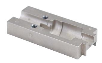
Fitel compatible, Metal, Splice-on Connector holders are specifically designed to fit the Fitel S123, S153, S178, S179, and NINJA model fusion splicers. Use this to hold the connectors inside the splicer when terminating Infinium splice-on connectors to ensure proper fusion splicing
