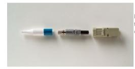
Legrand quick-cure, anaerobic epoxy field-installable connectors speed installation time. Strip the fiber, inject the adhesive into the connector, insert and scribe the fiber, then polish the connector end face to perfection for a high performance termination. Individual pack.
