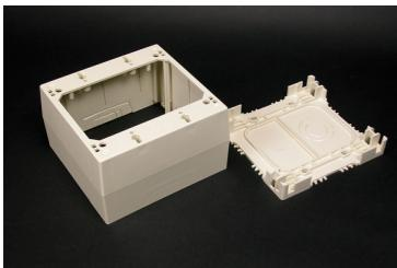
Two-gang. Base has rectangular K0 to enable extension from existing single-gang flush wall box and 1/2" and 1" trade size concentric K0s. Accepts industry standard faceplates for switch and communication devices.
