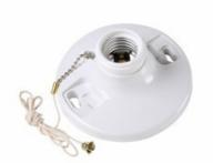
Medium base, phenolic, pullchain, 4 terminals with Tamper-Resistant-drive screws, fits 3 1/4 and 4-inch boxes, with cage necks.
