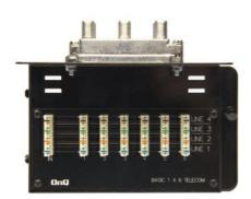
Supports telecom distribution to outlets via 110-style punchdown connections and video distribution. Does not include telecom surge protection, telecom expansion or security system interface.  $5\ 1/8$ ""H x  $6\ 1/2$ ""W
