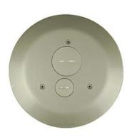
Complete with one-piece finish flange and conduit assembly. Conduit assembly consists of one 3/4inch trade size conduit and one 1 1/2inch trade size conduit. Finish cover flange provided with one 3/4inch trade size screw plug opening and one 1 1/2inch trade size screw plug opening. Covers available in painted black (BK), gray (GY), brass (BS), bronze (BZ), and brushed aluminum (AL). NOTE: Assembled with scrub water gasket. For use on tile, wood or carpet floors.
