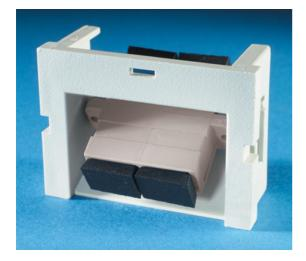
Series II Module, 1-SC Duplex (2 fibers) multimode adapter with phosphor-bronze alignment sleeves, innie. 60degree exit (1.5 units) 9 most popular line - It has the widest selection of interfaces, surface mount boxes and faceplates. Series II Modules use a 110 punch down sequence that is almost three times faster than other methods. The wide selection of multimedia modules include blanks for future growth
