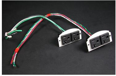
Two (2) proprietary 20A duplex power receptacles with mounting plates. Designed to fit in either of the two side compartments in both the 6ATC and the 8ATC Series Poke-Thru Devices. Receptacle can be wired as a standard or isolated ground device.
