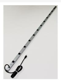
Twelve outlets, 6' (1.8m) cord. Length 77" (2m). Receptacle center-to-center 6" (152mm). 15 Amp unit with a 15A resettable circuit breaker.
