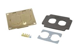
Brass duplex cover plate, for OmniBox® and Modulink™ Series floor boxes. Cover plate is 3.156 inch x 4.182 inch (80.2mm x 106.2mm). Flip lids can also be used with 106 type frames for communications. NOTE: Brass covers and flanges are not interchangeable with aluminum or nonmetallic covers and flanges. Nonmetallic covers are interchangeable with aluminum flanges.
