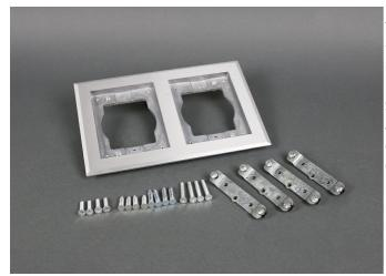
Two gang brushed aluminum combination carpet and tile flange, for OmniBox® and Modulink<sup>™</sup> Series floor boxes. Flange is 5.940 inch x 9.045 inch (150.9mm x 229.7mm). Accepts Ortronics MAB6TJ TracJack and MAB3S2 Series II, and Wiremold CM Series Open System adapters, sold separately. NOTE: Brushed aluminum flanges come with beveled edges. Brass cover plates can only be used with brass flanges. Brushed aluminum flanges come with beveled edges.
