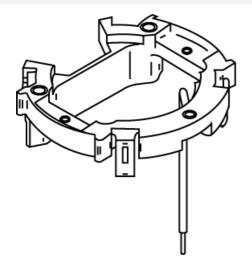
Used to attach wiring devices and cover plates to PVC box. Locks into place without using glue or mechanical fasteners. Compensates for up to 10° of tilt if box is not level. Ground wire is factory attached to the adjusting ring. One ring required per box, single- or dual-service, ordered separately.
