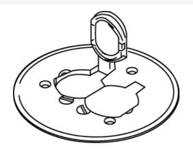
The Wiremold Ratchet-Pro™ brushed aluminum duplex cover plate with flip lids, 5 1/2 inch (140mm) for carpet or tile installations. Cover also works with 880 Series™ boxes. NOTE: All cover plates are furnished with gasket and three screws. The 895P Polycarbonate Series Cover Plates must be field modified for dual service.
