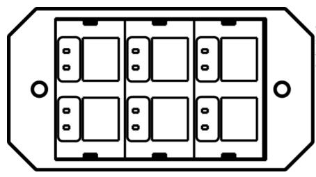
Single-gang device plate that will accept up to six (6) ports of communication devices. Fits in any one (1) of the three (3) gangs in the center compartment. Devices supplied by others.
