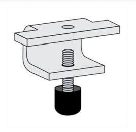
Now it is easy to connect wire mesh cable tray to ladder tray without drilling mounting holes.
