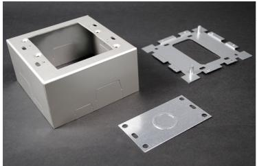
Two Gang Deep Device Box. For larger receptacles and deep devices such as those of signal and alarm systems. Base has open black plate for mounting to existing wall box and solid black plate insert with 1/2" and 3/4" trade size Kos to close opening. Accepts industry standard faceplates for communication devices. Aluminum
