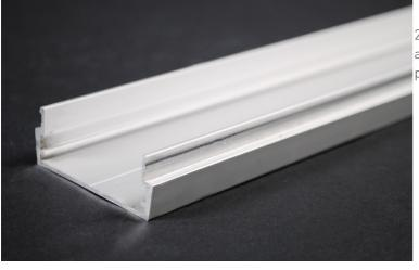
2" (51mm) wide, 6063-T5 extruded aluminum, satin anodized finish, .60" (1.5mm) nominal thickness. Base packed (12) 5' (1.5m) lengths per carton.
