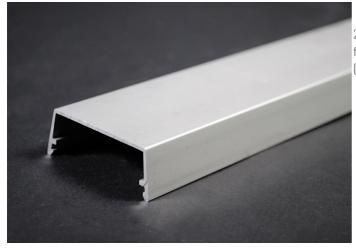
2" (51mm) wide, 6063-T5 extruded aluminum, satin anodized finish, .60" (1.5mm) nominal thickness. Cover packed (12) 5' (1.5m) lengths per carton.
