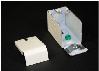
Connects 2000 Series Raceway to 1/2" trade size conduit or armored cable connectors. 1/2" trade size KOs located on end, sides, and bottom of fitting. Includes ground screw. If more capacity is required, use 2010A3.
