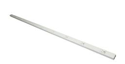
The Wiremold 2000 Series raceway offers a selection of steel, aluminum, and nonmetallic raceways that provide a versatile solution for many applications. Plugmold sections offer single or alternating circuits, in standard or isolated ground receptacles. The ScuffCoat finish is scratch resistant and protects against nicks and chips while preventing color from fading.
