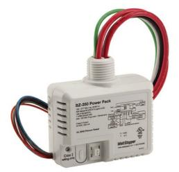
The BZ-250 power pack switches lighting or plug loads On and Off in response to low voltage control inputs, and provides up to 225mA at 24VDC to power Wattstopper occupancy sensors. It enables Manual-On sequences of operation, as well as HoldOn, Hold-Off and load shed applications when used with lighting control panels or building automation systems. This device is constructed with environmentally friendly materials and is RoHS-compliant.
