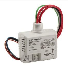
The BZ-250 power pack switches lighting or plug loads On and Off in response to low voltage control inputs, and provides up to 225mA at 24VDC to power Wattstopper occupancy sensors. It enables Manual-On sequences of operation, as well as HoldOn, Hold-Off and load shed applications when used with lighting control panels or building automation systems. This device is constructed with environmentally friendly materials and is RoHS-compliant.
