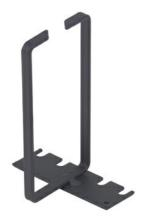
CR-93S-1B and CR-93S-3B rings fit within the width of a rack; they are designed for smaller, single-rack installations or where the width of the rack cannot be exceeded. Larger capacity CR-93S-2B and CR-93S-4B rings mount between adjacent racks and equal the combined width of the rack channels; they are designed for multiple rack installations
