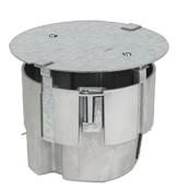
The CRFB2 Floor Box is a 2 compartment round recessed housing designed to accommodate power, communications, and audio/video services for raised and wood floor applications. Popular aplications for the CRFB floor box include: open office environments, conference rooms, computer centers, stages and altars. The CRFB Series floor box can accept the 6" Evolution Series Poke-Thru Device covers and are available in six aesthetic colors: black, gray, brass, nickel, bronze, and aluminum.
