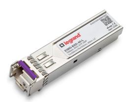
Brocade E1MG-BXD-40 Compatible 1000Base-BX SFP Transceiver (SMF, Tx: 1490nm Rx: 1310nm, 40km, LC Duplex, DDM, I-Temp)
