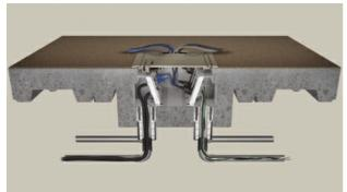
6-Gang Fire Classified Floor Box. Pre-assembled installation ready Floor Box has been designed to be installed in above grade concrete floors while maintaining the fire classification of the floor. This box is classified to be used in 1-, 1 1/2-, 2-, or 3-hour fire rated floors. Designed to accept standard size wall plates. Box comes complete with all components needed for initial installation.
