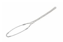
FC050U: Standard Duty, Closed Mesh, Single-Eye Grip, Cable Diameter 0.50 - 0.61 inches, Bale Length 7-in, Mesh Length 11-in, Break Strength 770 lbs.
