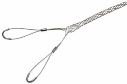
FC062UU: Standard Duty, Closed Mesh, Double -Eye Grip, Cable Diameter 0.62 - 0.74 inches, Bale Length 4-in, Mesh Length 11-in, Break Strength 1150 lbs.
