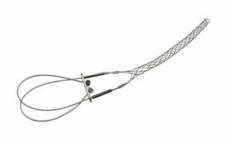
FC100LB: Standard Duty, Closed Mesh, Locking Bale (Universal Eye), Cable Diameter 1.00 - 1.24 inches, Bale Length 18-in, Mesh Length 15-in, Break Strength 1920 lbs.
