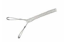
FC150UU: Standard Duty, Closed Mesh, Double -Eye Grip, Cable Diameter 1.50 - 1.74 inches, Bale Length 6-in, Mesh Length 18-in, Break Strength 1920 lbs.
