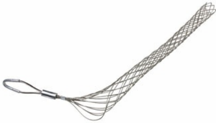
FC3000F: Standard Duty, Closed Mesh, Offset Eye Grips, Cable Diameter 3.00 - 3.49 inches, Bale Length 9-in, Mesh Length 26-in, Break Strength 5040 lbs.
