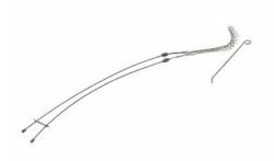
FR062LB: Standard Duty, Split Rod, Locking Bale (Universal Eye), Cable Diameter 0.62 - 0.74 inches, Bale Length 10-in, Mesh Length 9-in, Break Strength 1150 lbs.
