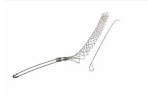
FR100U: Standard Duty, Split Rod, Single Eye, Cable Diameter 1.00 - 1.24 inches, Bale Length 9-in, Mesh Length 15-in, Break Strength 1680 lbs.
