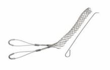
FR125UU: Standard Duty, Split Rod, Double-Eye, Cable Diameter 1.25 - 1.49 inches, Bale Length 5in, Mesh Length 16-in, Break Strength 1680 lbs.
