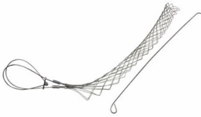
FR175LB: Standard Duty, Split Rod, Locking Bale (Universal Eye), Cable Diameter 1.75 - 1.99 inches, Bale Length 14-in, Mesh Length 17-in, Break Strength 3150 lbs.
