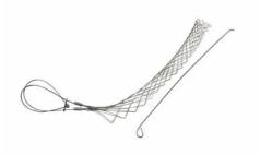
FR200LB: Standard Duty, Split Rod, Locking Bale (Universal Eye), Cable Diameter 2.00 - 2.49 inches, Bale Length 18-in, Mesh Length 20-in, Break Strength 3360 lbs.
