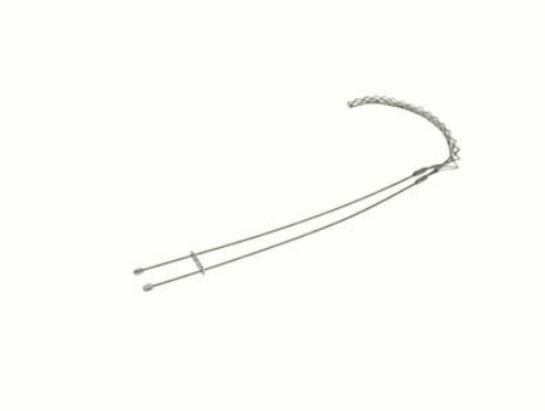
FS050LB: Standard Duty, Split Lace, Locking Bale (Universal Eye), Cable Diameter 0.50 - 0.61 inches, Bale Length 18-in, Mesh Length 11-in, Break Strength 770 lbs.
