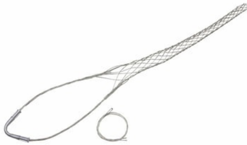
FS050U: Standard Duty, Split Lace, Single Eye, Cable Diameter 0.05 - 0.61 inches, Bale Length 7-in, Mesh Length 11-in, Break Strength 770 lbs.
