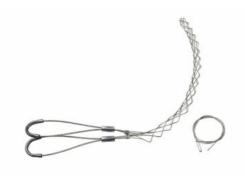
FS050UU: Standard Duty, Split Lace, Double-Eye, Cable Diameter 0.50 - 0.61 inches, Bale Length 4-in, Mesh Length 11-in, Break Strength 770 lbs.
