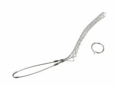
FS125U: Standard Duty, Split Lace, Single Eye, Cable Diameter 1.25 - 1.49 inches, Bale Length 10-in, Mesh Length 16-in, Break Strength 1680 lbs.
