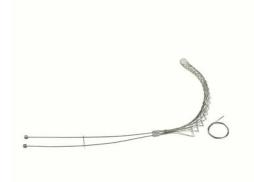
FS150LB: Standard Duty, Split Lace, Locking Bale (Universal Eye), Cable Diameter 1.50 - 1.74 inches, Bale Length 18-in, Mesh Length 18-in, Break Strength 1920 lbs.
