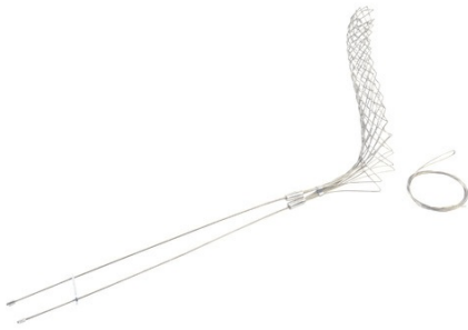
FS200LB: Standard Duty, Split Lace, Locking Bale (Universal Eye), Cable Diameter 2.00 - 2.49 inches, Bale Length 18-in, Mesh Length 22-in, Break Strength 3360 lbs.
