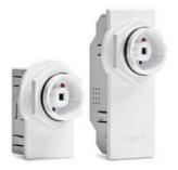
FSP-2x2 sensors provide multi-level control based on motion and/or daylight contribution. They control 0-10VDC LED drivers or dimming ballasts, as well as nondimming ballasts and, with an FSP-Lx Lens, are rated for wet and cold locations. Line and low voltage models are available, and choice of control modes simplifies sensor configuration.
