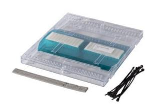
The 48-Fiber transparent fusion splice tray is ideal for fusion splicing single fiber. The see through cover and mylar insert enable easy viewing when visual fault locator (VFL) testing and verification is performed to ensure cable continuity and determine pass or failure of splicing. The hinged cover and carefully designed fiber routing enable quick and easy splicing and fiber management. The stackable design of this 7 inch tray, saves space while ensuring maximum density for the application.
