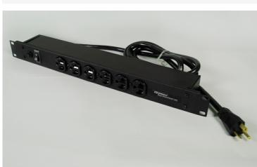
Six front 20A outlets, on/off switch, 15' (4.6m) cord. Receptacle center-to-center 1 1/2'' (38mm).
