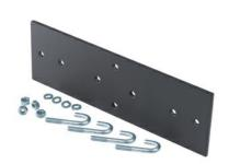
Used for junctioning cable runway and equipment racks. Runway can be junctioned parallel or perpendicular to rack. Cable runway mounting brackets mount to the top of the cabinet and provide a surface for attaching 6 in, 12 in, 18 in or 24 in W runway.
