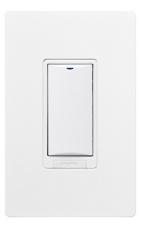
The LMDM-601 Dimming Wall Switch is a wireless low voltage device for dimming control of one or more lighting loads. It is part of the wireless Digital Lighting Management (DLM) system and can dim load(s) connected to wireless DLM dimming room controllers (LMRC-611) for a totally wireless room. Alternatively it can be used in a hybrid wired & wireless room to control loads connected to a traditional wired room controller (e.g. LMRC-111) when used in conjunction with a wireless bridge (LMBC-650).
