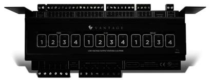
The Low-Voltage Output Station (LVOS) is used for the control and automation of LED, CFL, and CCFL lighting loads requiring either 0-10 or pulse width modulation (PWM) for dimming control. The dry contact inputs can be used with motion sensors, light sensors, pressure sensors, IR inputs, magnetic switches, and more. As part of the Legrand lighting solution, it provides control of LED loads as well as inputs from dry contacts for lighting and automation.
